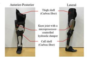
Figure 2: C-Brace consists of a carbon fiber thigh/lower leg shell made for each patient and a uniaxial knee joint with a computer-controlled hydraulic damper connected to it.
